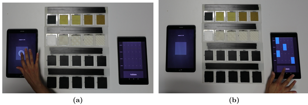
Figure 5.6 – Evaluation of a virtual sample with the tactile chart. (a) The virtual sample is explored. (b) Four answers from 1 to 5 situate the effect on the tactile chart.
